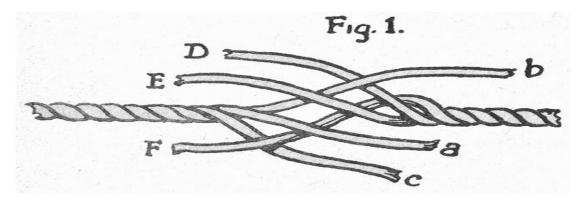
Starting with any one of these, lift it over its nearest neighbour in the married rope and then tuck it under the next in line, in the direction opposite the rope's natural twist. This is called *working against the lay*.
